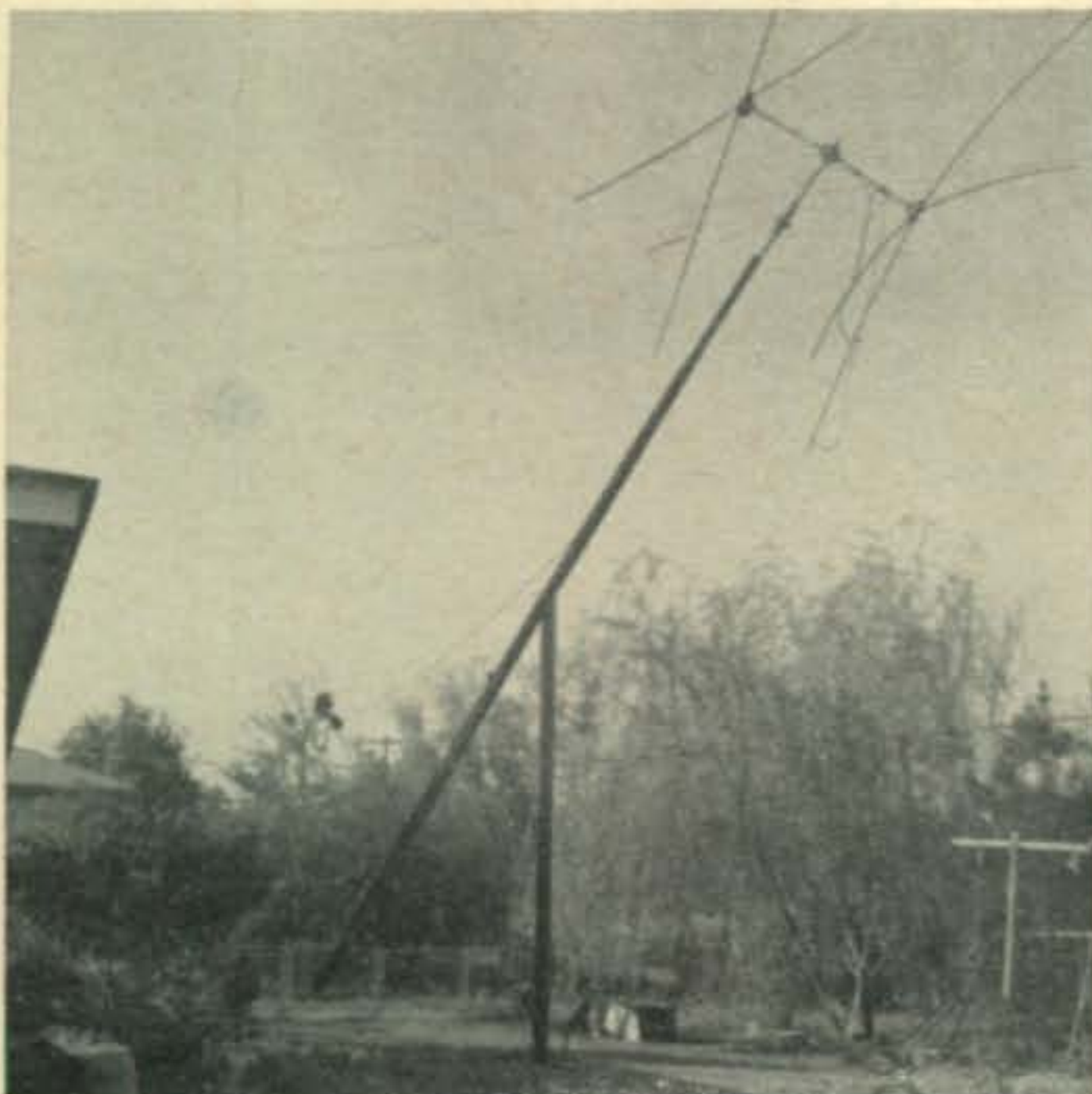
View of the cubical quad atop the partially tilted tower.
